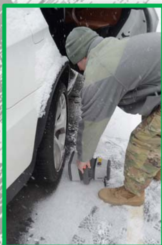
BELOW: SGT Vanderwerken scans the rear tire of the vehicle in question with the Mini-Z scanner.
