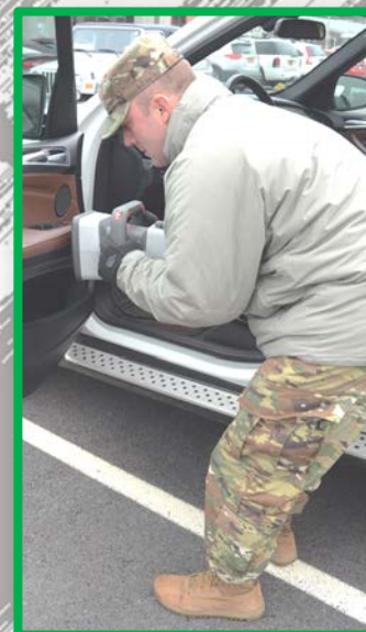
ABOVE: CPL Long scans the driver side door of the confiscated SUV with the Mini-Z scanner. Ensuring nothing was missed during the LEA search of the vehicle earlier in the week, CPL Long makes sustained sweeps with the scanning device that then shows a printable image on the hand held screen. The Mini-Z scanning system is a scanner that is accompanied by a hand-held screen.
