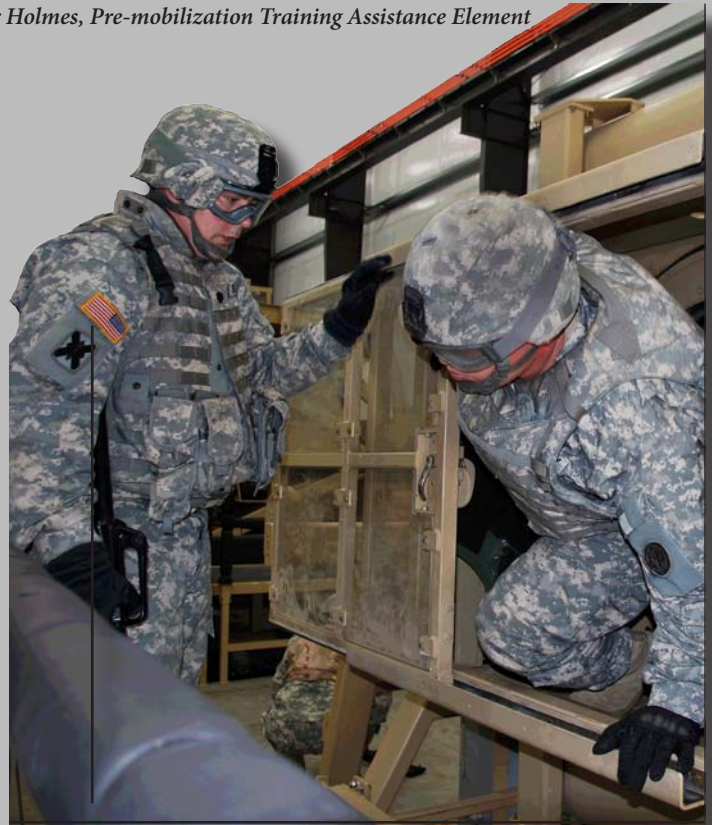
27th Infantry Brigade Combat Team Soldiers get certified on the Humvee Egress Assistance Trainer as part of their pre-deployment training. The HEAT trainer closely replicates a humvee that has rolled over, forcing Soldiers to escape individually and assist everyone in the vehicle until everyone is accounted for. Photo by Sgt. 1st Class Raymond Drumsta, 27th IBCT.
