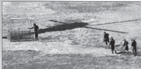
Volunteers from the 106 th Rescue Wing move to board (above) and ride on (below) a rescue basket during its certification testing.
