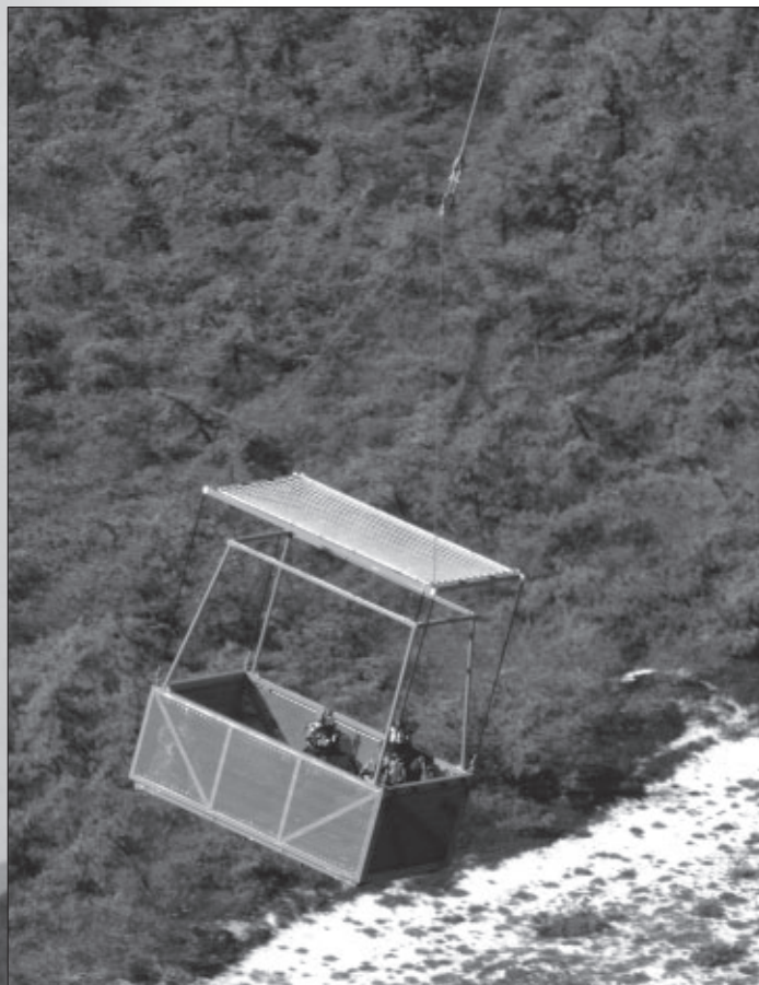
Volunteers from the 106 th Rescue Wing move to board (above) and ride on (below) a rescue basket during its certification testing.
