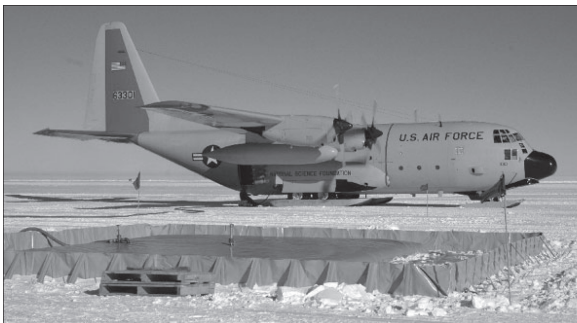
A 109 th Airlift Wing LC-130 Hercules refuels from a fuel bladder on an ice runway in Antarctica.
