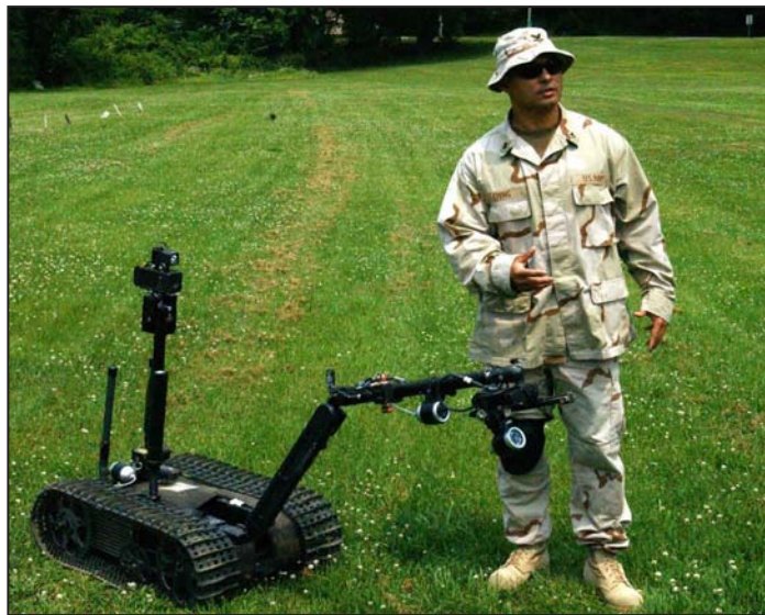
Navy Petty Officer 2nd Class Joseph Ching, Space and Naval Warfare 220, from San Diego, Calif. prepares the Talon Mark 4 Explosive Ordnance Disposal robot for a demonstration. The robot is used to investigate and destroy improvised explosive devices in Iraq and Afghanistan. Ching is part of an active-duty ordnance training team visiting Camp Smith to provide training for New York's 501 st Ordnance Battalion (EOD) and 1108 th Ordnance Company (EOD), headquartered in Schenectady.
