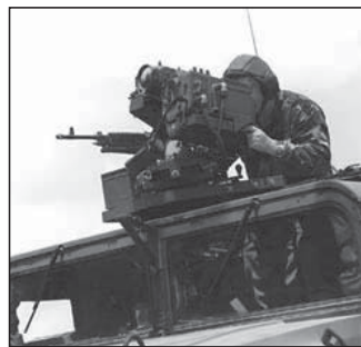
The M707 Knight is a precision targeting system consisting of a laser designator/rangefinder, thermal imager, digital command and control, blended inertial/GPS navigation and targeting, and a self-defense weapon. The system fielding was part of the N.Y. National Guard logistics synchronization conference held at Fort Drum September 27-28, 2006. DoD image.
