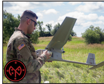
Cpl. Matthew Mena, a field artillery tactical data specialist assigned to Charlie Battery, 1st Battalion, 258th Field Artillery Regiment, prepares an RQ-11B Raven unmanned aircraft for flight at Fort Drum, New York, July 2019. The Raven, a small hand-launched aircraft, is utilized to conduct short range reconnaissance. Photo by Sgt. Alexander Rector, 27th Infantry Brigade Combat Team.
