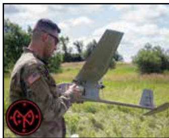
Cpl. Matthew Mena, a field artillery tactical data specialist assigned to Charlie Battery, 1st Battalion, 258th Field Artillery Regiment, prepares an RQ-11B Raven unmanned aircraft for flight at Fort Drum, New York, July 2019. The Raven, a small hand-launched aircraft, is utilized to conduct short range reconnaissance. Photo by Sgt. Alexander Rector, 27th Infantry Brigade Combat Team.
