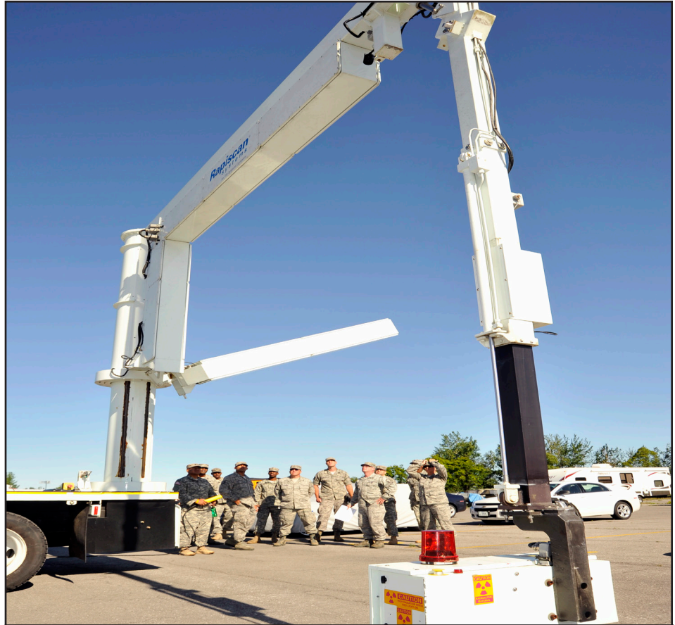
Members of the Counterdrug Task Force train on the Rapiscan system, which enables law enforcement agencies to search for hidden drug compartments in seized vehicles.
