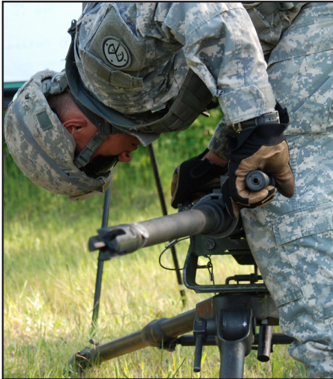
Sgt. Daniel Washburn of A Troop, 2nd Squadron, 101st Cavalry, demonstrates a feature of the M2A1 .50 Caliber machine gun that allows easier barrel changing.
