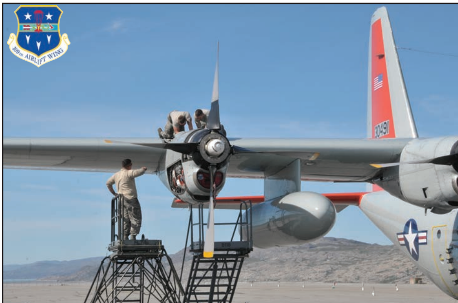
Above, Senior Airman Frank Pambianchi, Staff Sgt. Chris Holt, and Senior Airman Nathan Martineau, with the 109th Aircraft Maintenance Squadron, replace engine components on an LC-130 aircraft engine at Kangerlussuaq, Greenland July 27, 2017. At right, Master Sgt. Randy Powell loads a training pallet onto an LC-130 aircraft July 28. Powell is an instructor loadmaster, qualifying new crewmembers for polar operations. About 80 personnel from the 109th Airlift Wing and four LC-130 aircraft were deployed on the unit's fifth rotation for mission support in Greenland. The support season started in April and runs through September.
