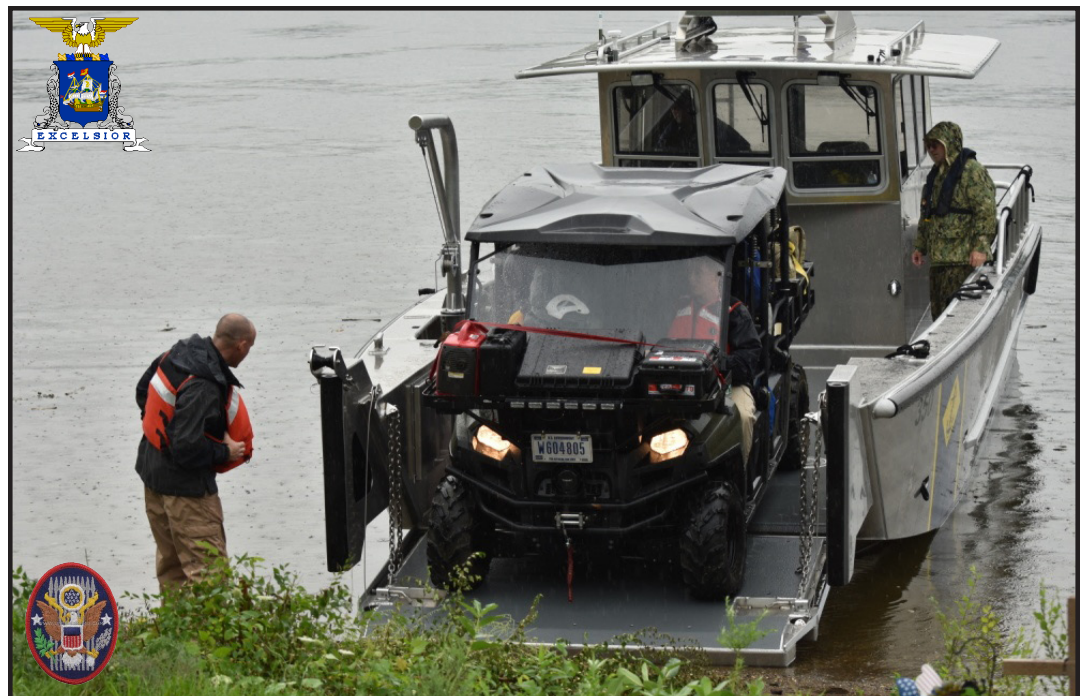
Members of the New York National Guard's 2nd Civil Support Team unload an ATV from the New York Naval Militia's new landing craft, LC-350, during a joint training exercise conducted on the Hudson River in Rensselaer, New York on August 17, 2018. The Naval Militia Sailors and CST members were testing the ability of the boat to load and unload the ATV, used by CST chemical, biological and radiological survey team members, on the shore. Photo by Spc. Andrew Valenza, Joint Force Headquarters.
