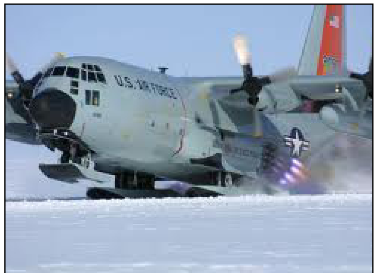
Archive photo of a 109th 'Ski Bird' taking off with a, then; jet-assisted takeoff rockets alongside. Since then, the aircraft uses an eight-blade propeller system for its Arctic takeoffs.
