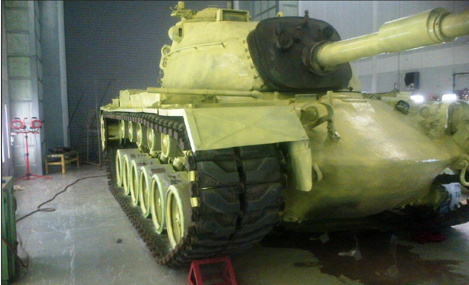
This M-48A5 tank, used by Army National Guard Armored Battalions in the 1970's and 80's, will be repainted by the New York Maneuver Area Training Equipment Site for display by the Connecticut National Guard as a historic vehicle. Courtesy photo.
